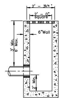
All precast concrete shall meet O.D.O.T. 706.13 requirement.
