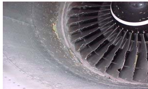
A gull caused the damage viewed on this engine.
